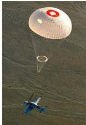
Ballistic Parachute Systems have an actuation T-handle (usually red) within reach of the pilot attached to a sheathed cable. The cable runs directly into the rocket igniter attached to the parachute container. In most cases, the parachute deploys up and aft, and the entire assembly is located close to the aircraft center of gravity; around where the wing and fuselage meet.
