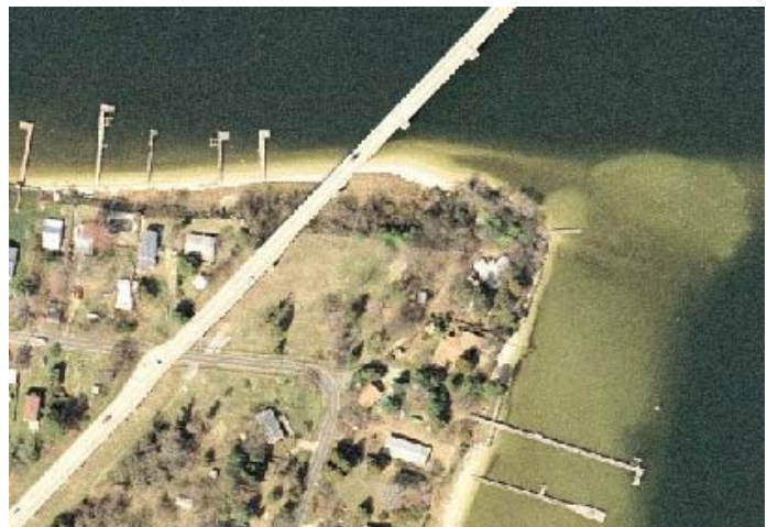
MD 4 (Patuxent Beach Road) shown above is currently a two lane roadway and serves as a major collector between St. Mary's County and Calvert County. This roadway is expected to operate at LOS F by the year 2025 unless the roadway and the Thomas Johnson Bridge are widened.
